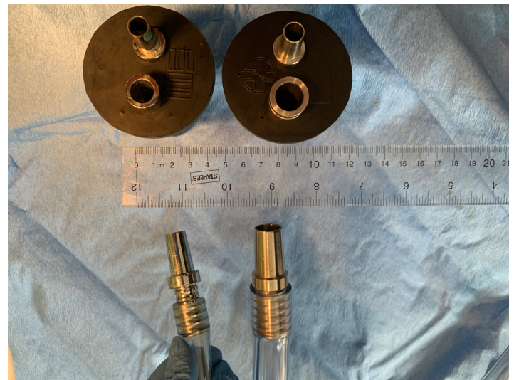
FIGURE 2: Regular (3/8") and Larger (3/4") tubes + tops for EVA machines
